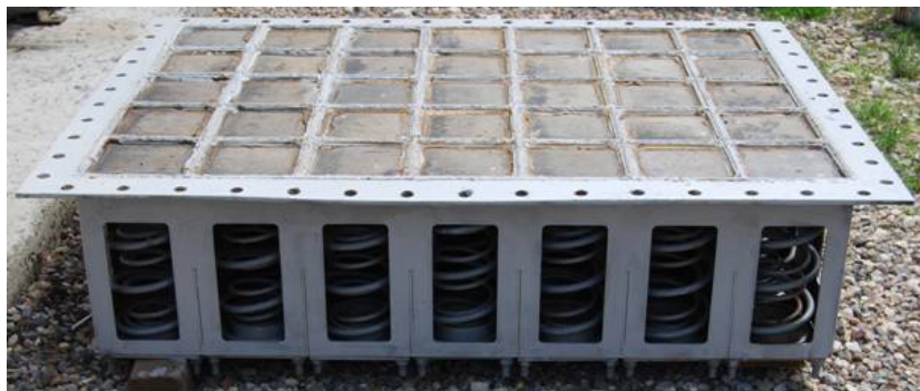
Figure 6 – Dynamic protection system (valve blocks without guard cover)
